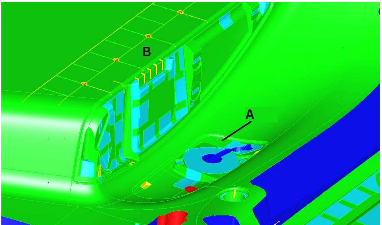
Fig.14 Different shapes require different strategies. Staying vertical for the floor “A” whenever possible and having the tool tipped at a constant angle for “B”.
