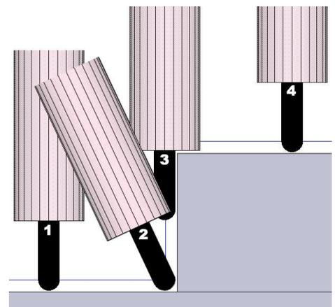
Fig.8 Collision free toolpath positions.
