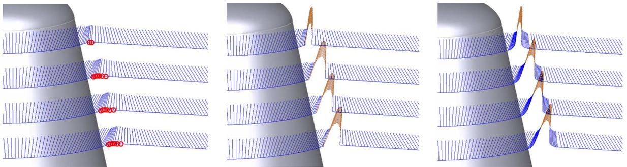
Fig.11 Marked collisions are replaced by vertical or radial movements.
