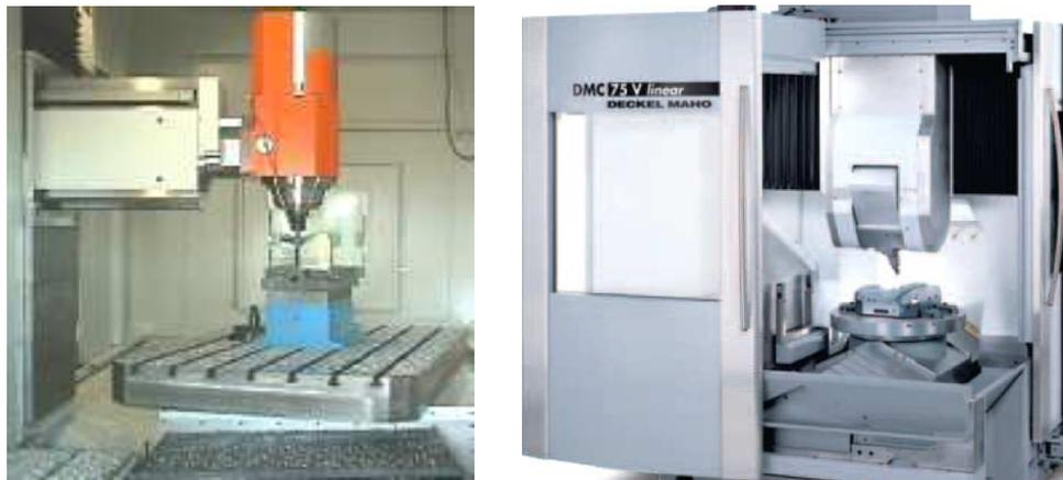
Fig.4 The 5-axis machines Auerbach IA 5 B and DMC 75V.
