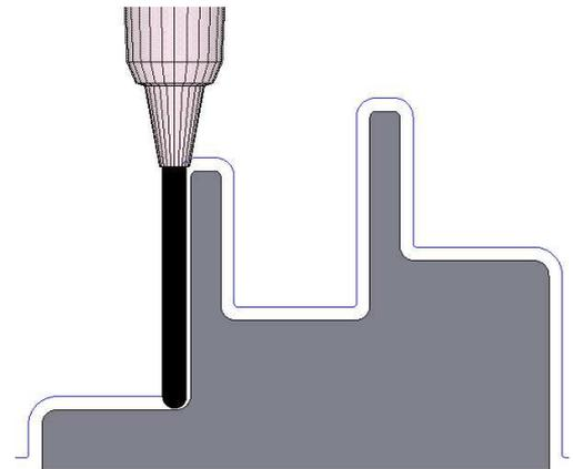
Fig. 1 3-axis toolpath.
