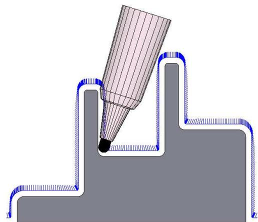
Fig.3 5-axis toolpath.
