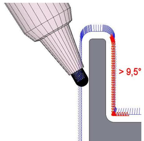
Fig.5 The angle limit of  $9.5^\circ$  will immediately stop DMC 75V.
