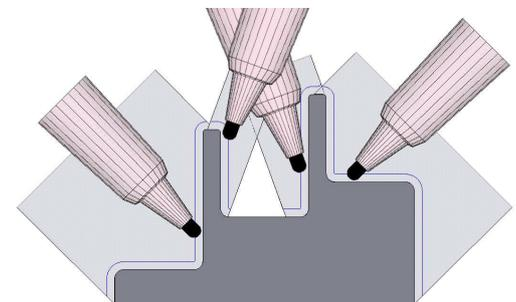
Fig.2 3+2-axis toolpath.
