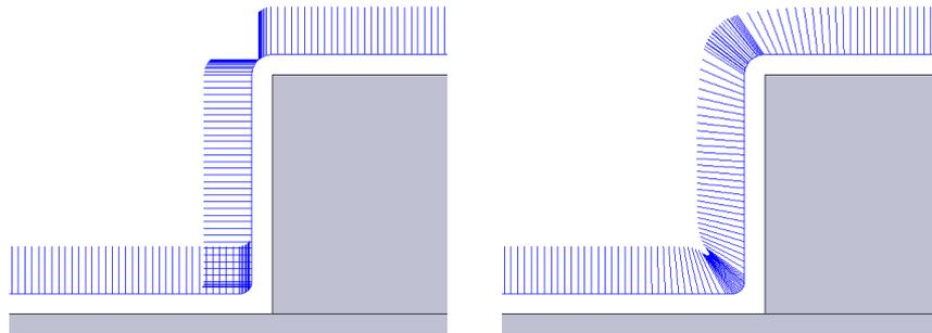
Fig.7 A normal to surface toolpath can usually not directly be machined.
