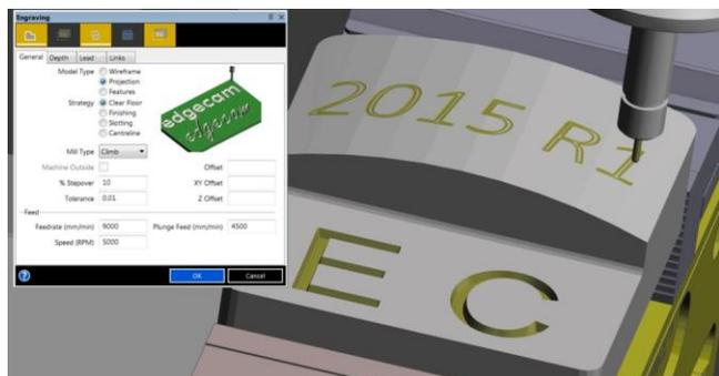
**New Engraving Cycle:** The new machining command ‘Engraving Cycle, allows complex geometry corners to be shaped, and artwork profiles to be machined. Using direct picking, the cycle works with a variety of entities, and offers four different types of strategies.
